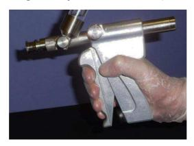
Another method is to fill the back of the injection head with solution using a syringe (this is the part of the head that is screwed to the device and is penetrated by the end of the plunger).
