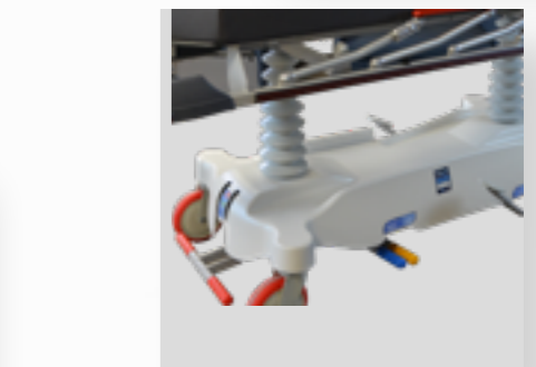
Two-sided head-end height adjustment and Trendelenburg / Anti-Trendelenburg adjustment
